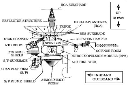
Demonstrate the difference between a body-mounted-instrument spacecraft like Cassini and a spacecraft with a scan platform like Galileo. This illustrates the difficulties presented to the Cassini science and engineering teams when they plan data collection using multiple instruments.
