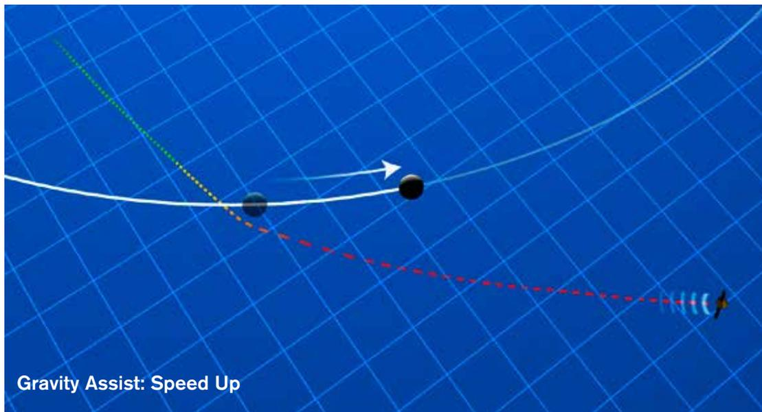
Examples of a spacecraft encountering a planet for a gravity assist. Depending on how the spacecraft approaches the planet, it will either speed up or slow down.
